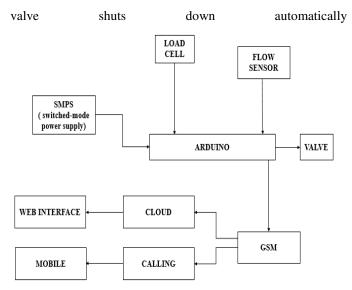
Figure 1- Block diagram for patient drip monitoring system
